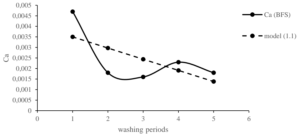
Figure 3. The dynamics of Ca migration from the soil limed with blast furnace slag (BFS)
